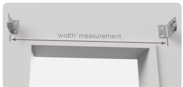
figure 4: outside fit bracket fixing
